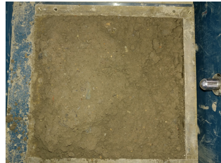
(b) The destroyed shear surface of the sample after testing
