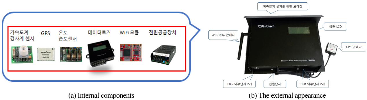
Fig. 4. Internal and external configurations of the instrument
